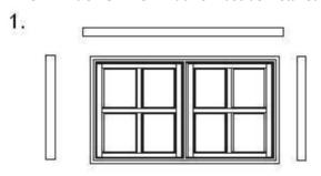
Place the window frame and four support trims on the stable surface.
