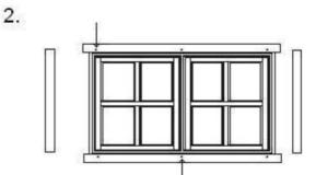
Drill the holes in the support trims and screw them in to the window frame.
