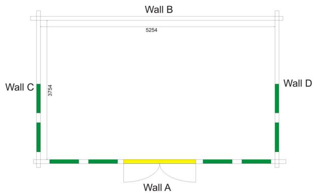
The wall-boards must be placed so that the ends interlock. Now screw the first row of wall-boards into the bearers. All the following rows of placed wall-boards should interlock not only at the ends, but along their length as well. Please screw each new row of wall-boards into the former row to ensure a solid structure.
