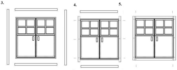
Then insert door frame in to its space from the outside of the structure. Finally attach the rest of the support trims to the door frame from the inside the structure.
