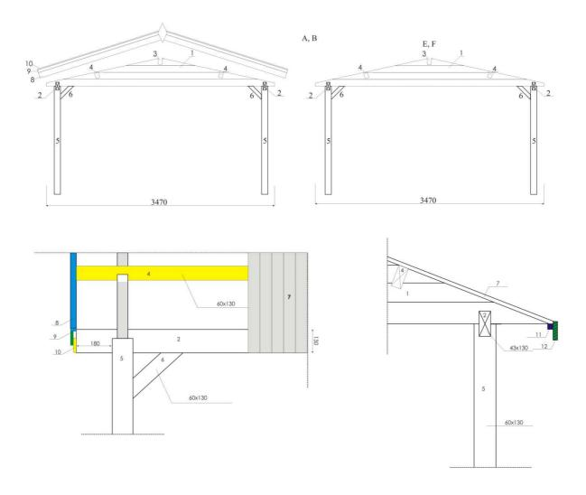
**4.4. Roof-boards:** Attach the roof-boards vertically and screw them into the rafters as shown in the page 3. Make sure the ends of the roof-boards are perfectly parallel to each other. Then fix the roof plank boarder under the roof-boards. The roof-plank must be screwed to the roof plank boarder.
