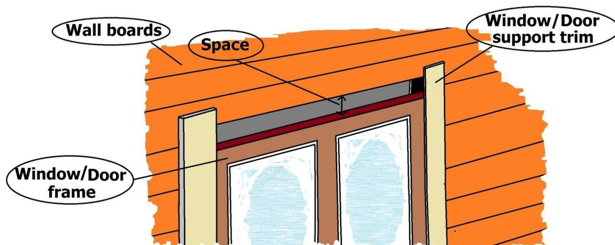
**4.10. Windows:** The windows must be installed in the same way as the door:
