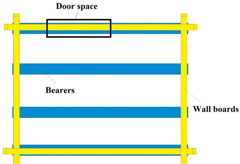
The wall-boards must be placed so that the ends interlock. Now screw the first row of wall-boards into the bearers. All the following rows of placed wall-boards should interlock not only at the ends, but along their length as well. Please screw each new row of wall-boards into the former row to ensure a solid structure.
