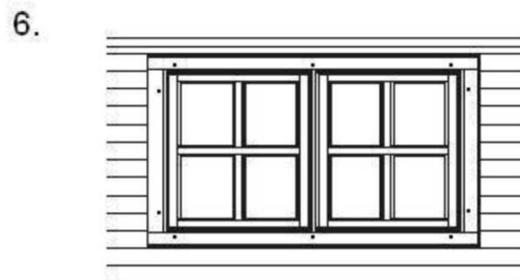
Now screw the rest four support trims in to the window frame from the other side.
