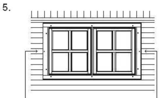
Just insert the window frame in to the space (no screwing)
