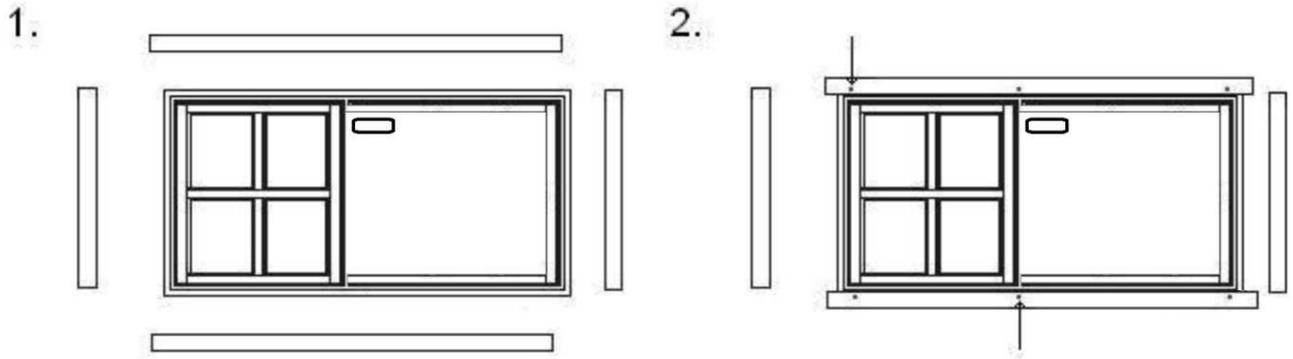
Insert door frame in to its space from the outside of the structure. Then fix the rest of the support trims from inside the building:
