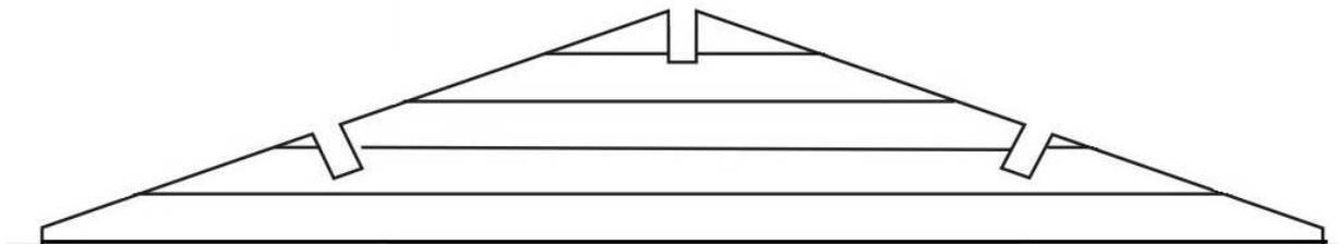
**4.6. Rafters:** The rafters must be mounted horizontally and inserted in the mounting-spaces found on the roof frame triangles. The rafters share a common mounting-space in the middle one of the three triangles. Here are two types of rafter-mounting shown below (picture)
