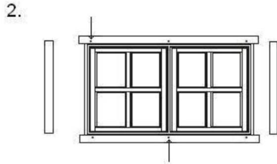
Drill the holes in the support trims and screw them in to the window frame.
