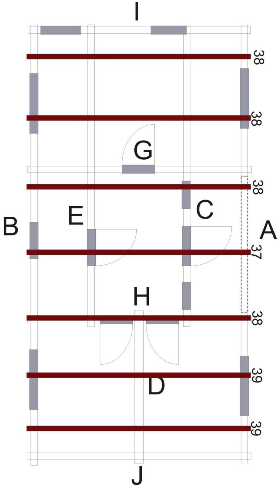
**4.7. Roof-boards:** The next step is to attach the roof-boards vertically and screw them into the rafters. Make sure the ends of the roof-boards are perfectly parallel to each other. Then fix the roof plank border under the roof-boards as show below. The roof-plank must be screwed to the roof plank border.
