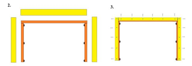
Then insert the door frame into place. The next step is to fix the rest of the support trims to the door frame from the other side. Notice: each frame support trim must fixed with at least 5 nails.
