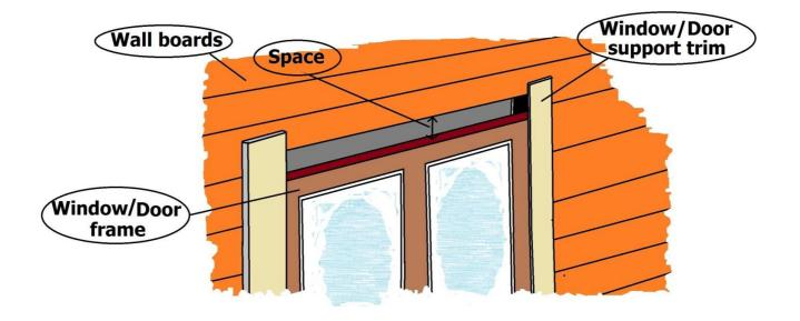
**4.10. Windows:** The windows must be installed in the same way as the doors:
