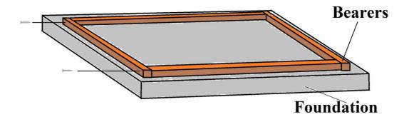
**4.4. Assembling the walls**: place the wall-boards directly on the bearers so that the wall-boards lay alongside them:
